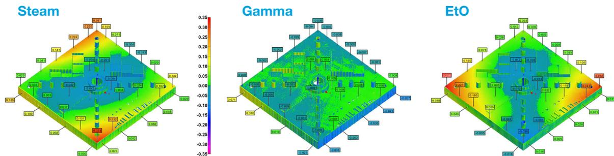
**Test 3:** After steam sterilization, models do not show a significant change in their mechanical properties. After Gamma and EtO sterilization, some changes are observed.
